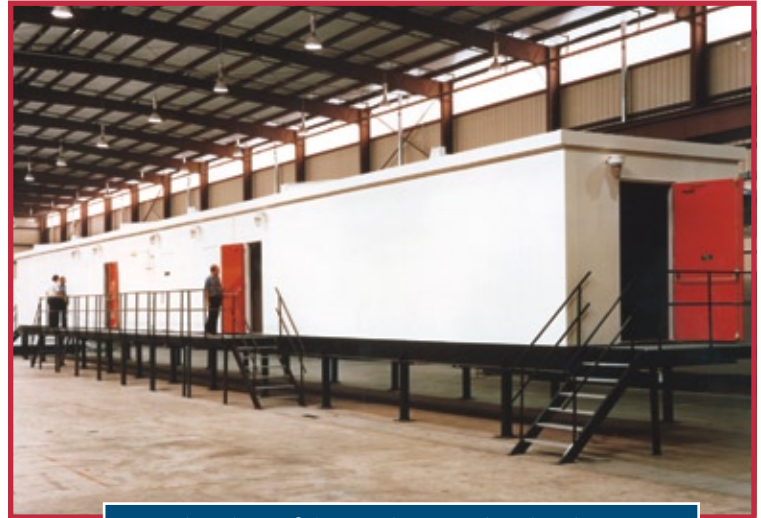
Completed PCR® (15' wide x 100' long) split across the width for shipment.
